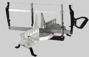
Mitre Saw Nobex Champion Compound Manual Mitre Saw. 630mm blade length; 125mm max. cap at 45°; 200mm max. cap. At 90°; 180mm max. cutting height; table size 500 x 125mm; blade width 45mm.
